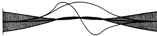
Fig. 11. The optimal design (form and cross-sectional area) of a clamped arch with c = 2 (and p = 3 ) for 0 \leq \bar{\alpha} \leq 0.07 (inactive constraint). The optimal frequency \omega = 77.6 is bimodal, and \omega/\omega_{cu} = 2.24 .
