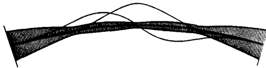
Fig. 5. The optimal design of a clamped circular arch with c = 6 (and p = 3 ) for 0 \leq \bar{\alpha} \leq 0.40 (inactive constraint). The optimal frequency \omega = 78.7 is bimodal, and \omega/\omega_{c_u} = 1.28 .
